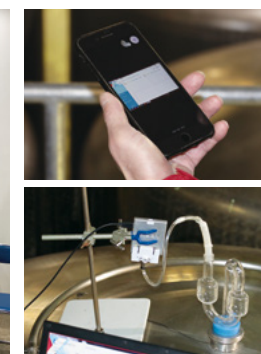
Using a wireless device to confirm wine fermentation progress and aroma constituents via smell sensors
